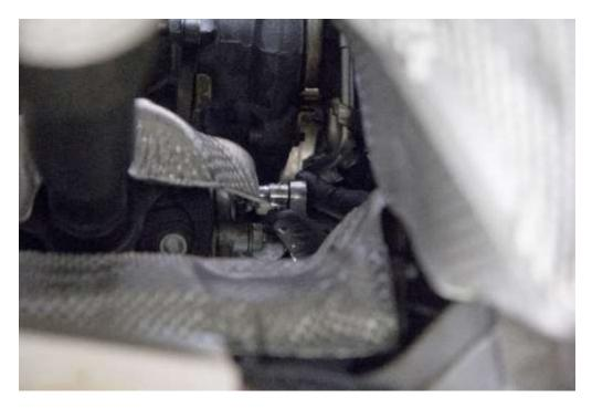
**Step 3:** Use your 21mm socket to undo the dogbone mount bolt and set aside.
