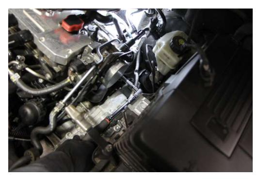
**Step 8:** Using your 13mm socket, remove the downpipe hanger bracket from the subframe.
