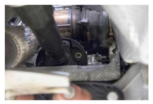
**Step 5:** Use your 22mm wrench to remove the secondary 02 sensor from the OEM downpipe.
