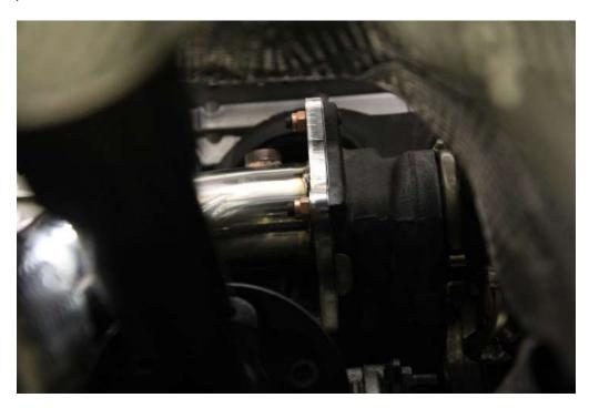
**Step 13:** Slide the 2 remaining downpipe sections into place and secure the 2 joints with the supplied accuseal clamps.
