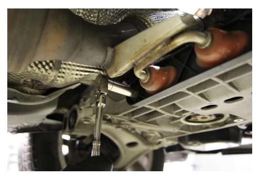
**Step 9:** Using your 13mm socket, undo the 2 bolts holding the OEM exhaust clamp to the catback. Slide the clamp towards the rear of the vehicle. Manuver the downpipe down and out of the vehicle.
