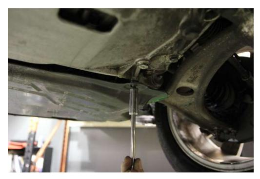
**Step 2:** Use your 10mm socket to remove 2x 10mm bolts holding the driveshaft heat shield in place. Pull the heat shield free of the car. This will <u>not</u> be reattached.
