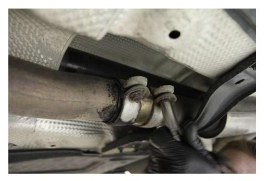
**Step 10**: Use your exhaust hanger removal tool and transfer the hanger from the OEM downpipe to the CTS downpipe.
