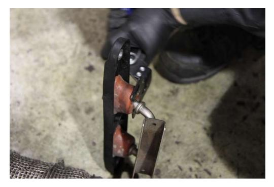
**Step 11**: Place the gasket over the turbine housing studs. Gasket is included in the optional install kit.
