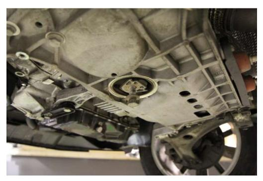
**Step 4:** Using the 10mm 12 point, remove the 3 bolts attaching the driveshaft to the transmission. Spin the 2 front wheels together to rotate the driveshaft allowing access to each bolt. Pull the driveshaft towards the rear of the vehicle and off of the flange. Push to the right side.
