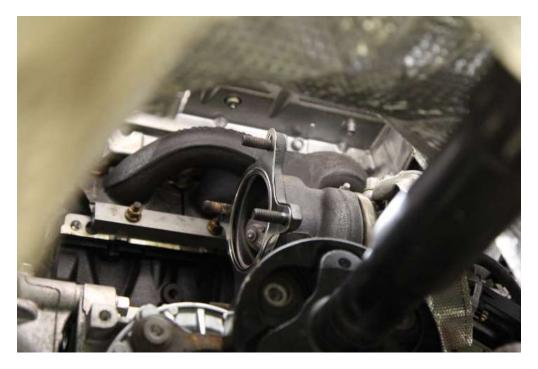
**Step 12:** Install the CTS downpipe and use new copper locknuts. Locknuts included in install kit (optional).
