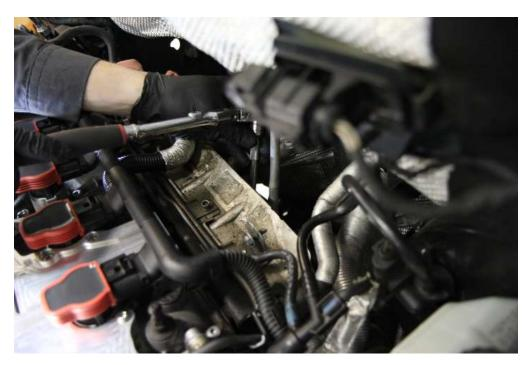
**Step 7:** Using your 16mm socket and extension, align your tool as shown to remove the upper forwardmost downpipe nut. Remove the 2<sup>nd</sup> upper nut as well. Move to the bottom of the car to remove the lower 2 retaining nuts.
