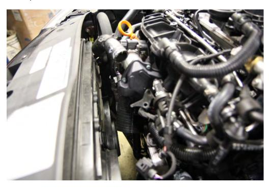
Step 11: Place the second hose clamp loosely over the top of the throttle pipe and feed the pipe up from the bottom inserting it into the upper silicon hose. Tighten the hose clamp over the silicon and pipe joining the throttle pipe to the throttle body.
