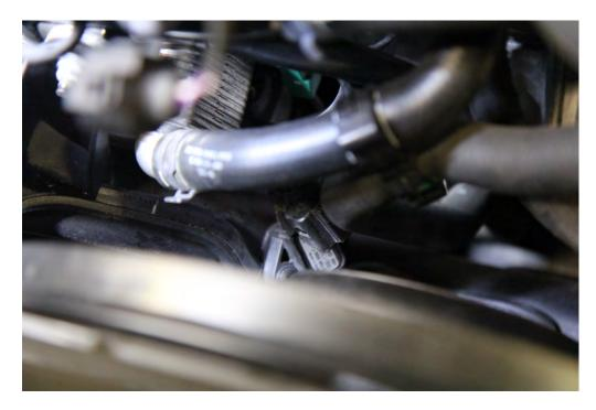
Step 4: Using a ratchet with a 10mm socket, undo the bolt holding the top bracket of the throttle pipe to the engine.
