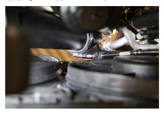
Step 12: Using the T30 Torx bit, reattach the bottom bracket of the throttle pipe to the engine.
