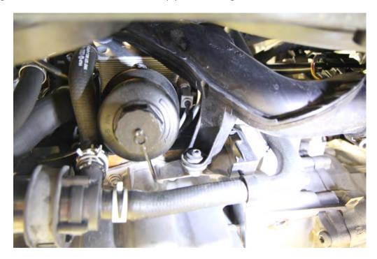
Step 6: Using a flathead screwdriver or 8mm socket, loosen the 2 hose clamps holding the rubber hose to the bottom of the throttle pipe and the intercooler. Pull the hose free.
