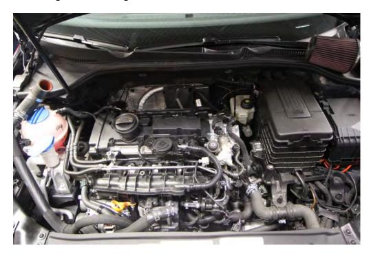
Step 2: Using a ratchet with an 8mm socket, loosen the 2 hose clamps at the top of the throttle pipe connecting it to the throttle body. (Golf R OEM pipe seen here).
