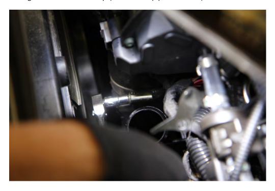
Step 3: Pull the connector off of the the MAP sensor located halfway down the stock throttle pipe.
