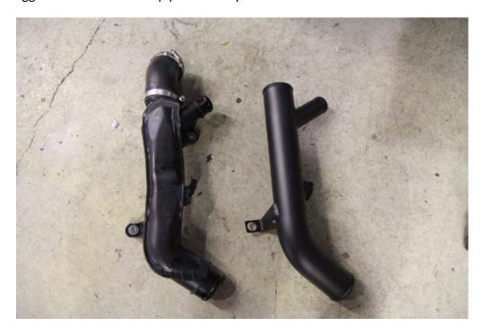
Step 8: Transfer the bottom mounting bracket hardware (rubber bushing with metal sleeve) to the new throttle pipe. Using a Philips screwdriver, remove the MAP sensor off the old pipe. Reattach to the new pipe using an 8mm socket and the supplied bolts.
