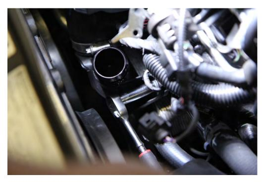
Step 5: With the car up on a hoist or on jackstands. Use a T30 Torx bit to remove the bolt holding the bottom bracket of the throttle pipe to the engine.
