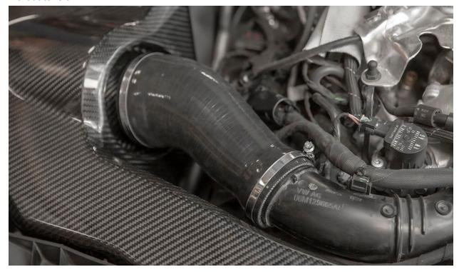
When you are happy with the silicone position, use a screwdriver to tighten both hose clamps firmly. *Do not overtighten hose clamps*.
