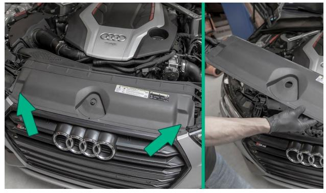
Pull up to release and remove the engine cover.
