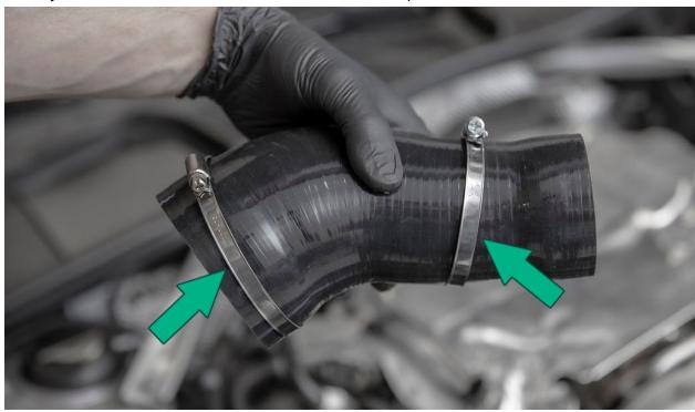
Install the silicone inlet between the IE intake velocity stack and the turbo inlet pipe. Adjust inlet and silicone positions as needed, make sure nothing is pulling or bound, and that it sits freely without tension.
