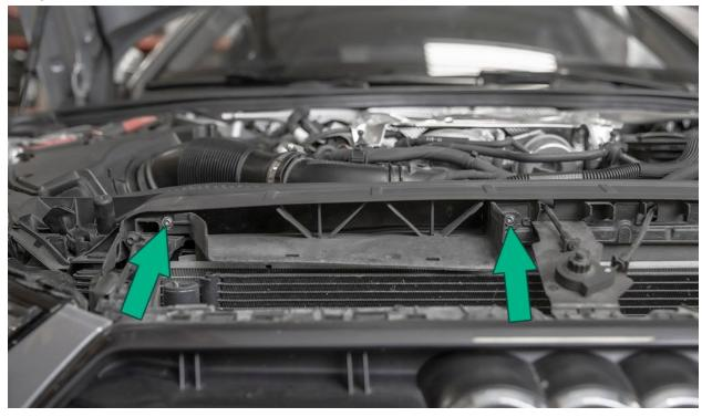
Pull up to disconnect and remove the intake snorkel.
