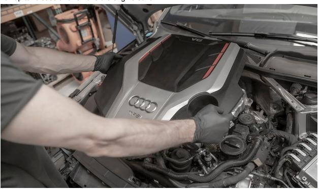
Using a T20 Torx driver, remove booth intake snorkel screws from the radiator support.
