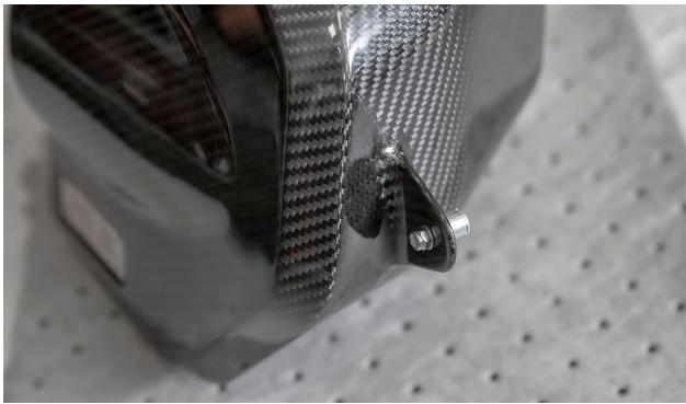
Press the factory grommet mount onto the mounting pin assembly.
