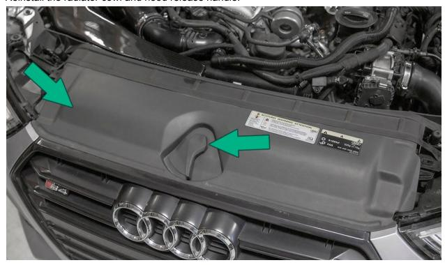
Line up the engine cover mounts and press firmly to reinstall.
