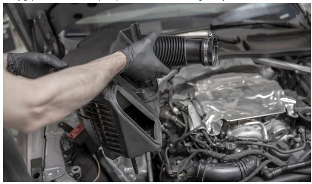
Pull the factory mounting grommet off the intake box and set it aside, it will be used for the installation of your new intake.
