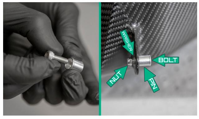
Using an 8mm socket and 4mm Allen, firmly tighten the grommet mount pin assembly. *Do not overtighten, this could crack the carbon fiber.*
