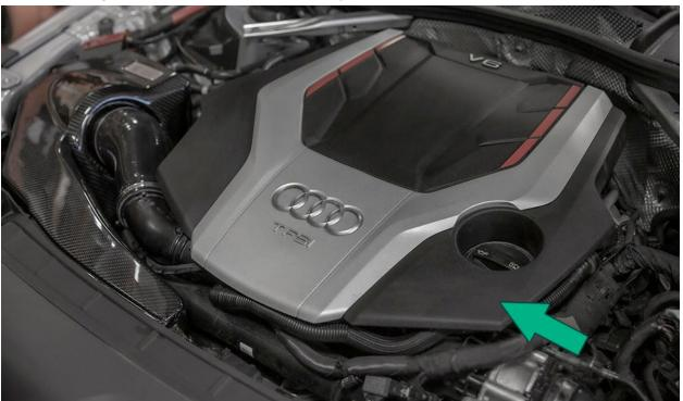
Verify all hose clamp connections are tight, and that your intake is fully installed. Start the car and inspect for any leaks or rubbing components.
